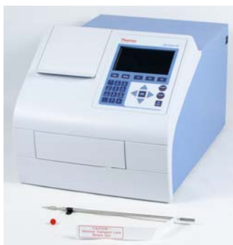
Figure 3–10. Transport lock removed
