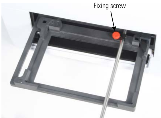
Figure 3–9. Plate carrier pulled fully out
