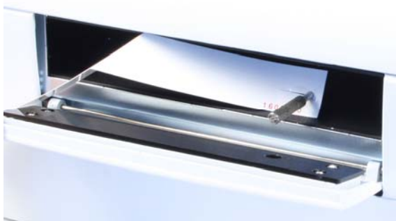
Figure 3–8. Transport lock bar with warning tag
