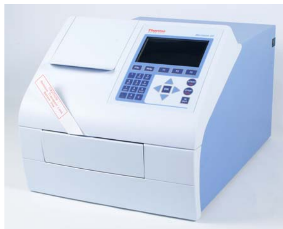
Figure 6–19. Multiskan GO with the transport lock in place
