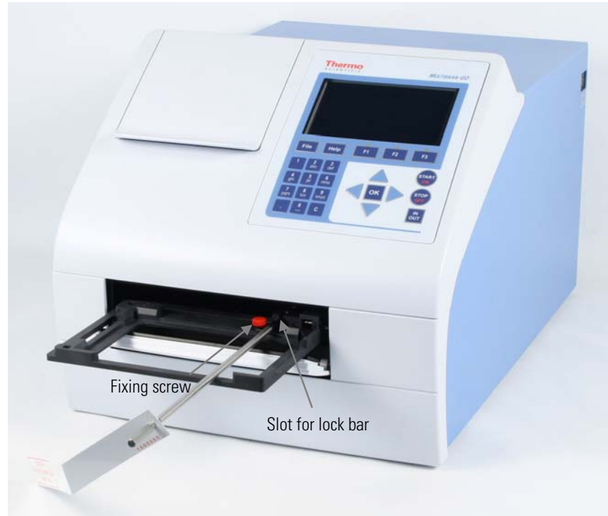
Figure 6–18. Transport lock bar in place on plate carrier
