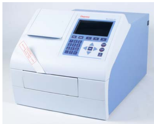
Figure 3–7. Multiskan GO with the transport lock in place
