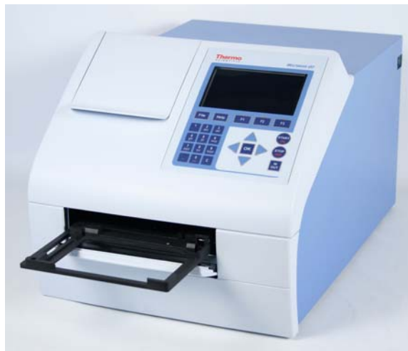
Figure 6–17. Plate carrier fully out of the instrument
