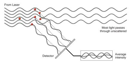
The scattered light falling on the detector.
