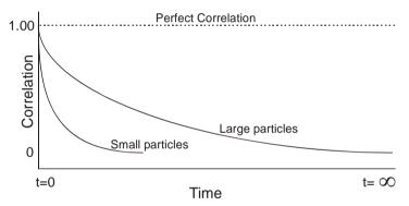
After the correlation function has been measured this information can then be used to calculate the size distribution. The Zetasizer software uses algorithms to extract the decay rates for a number of size classes to produce a size distribution.
