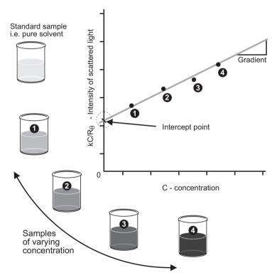
As only one measurement angle is used in this case, a plot of  $KC/R_{\theta}$  versus C should give a straight line whose intercept at zero concentration will be 1/Mw and whose **gradient** is proportional to  $A_2$ .
