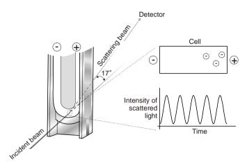
The light scattered at an angle of 17° is combined with the reference beam. This produces a fluctuating intensity signal where the rate of fluctuation is proportional to the speed of the particles. A digital signal processor is used to extract the characteristic frequencies in the scattered light.
